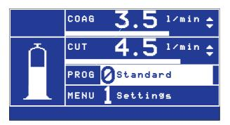
After selecting the PROG field, pressing the ENTER button shortly will open a submenu.
