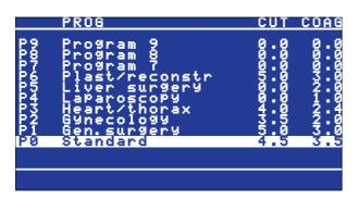
To storage positions P0 to P6, plain-text names and specific settings have already been preassigned in the factory. Note, however, that these settings are only recommendations. The user can of course change or completely overwrite them at any time!
