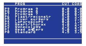
At the end of the name field, the cursor will jump to the CUT gas flow field upon pressing the SELECT button. Here, the CUT gas flow rate value can be changed with the  $\uparrow$  and  $\downarrow$  buttons as appropriate and in the same manner as in the main menu and will be kept stored permanently.
