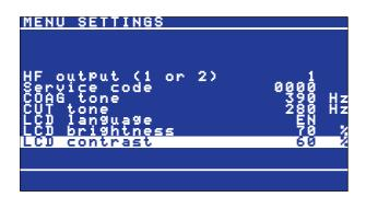
**Brightness:** Sets the light intensity of the screen. The primary light source of the screen is a fluorescent lamp subject to normal wear and tear. This means that the useful life of this lamp depends on the selected brightness level: the higher the brightness, the shorter the lamp's life. If the lamp cannot be ignited any more, the screen will remain dark and the lamp must be replaced.
