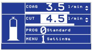
If the coagulation or cutting function is activated, the corresponding menu field (i.e. all of it) is displayed inversely and an activation signal is sounded. During activation, the gas flow rate can be adjusted with the  $\uparrow$  or  $\downarrow$  button if required, while the SELECT and ENTER buttons are inactive (function blocked) in the main menu in this case. Activation is also possible, however, when a submenu has been called up.
