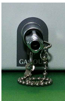
Fig. 3 Luer adapter for connecting a male Luer connector to socket 2, Fig. 2
