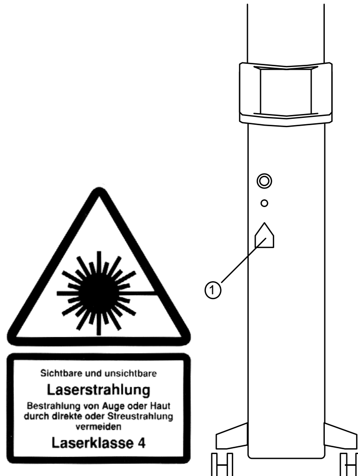
Fig. 2.1 1 "Laserstrahlung" (Laser Radiation) and "Laserklasse" (Laser Class) warning labels according to DIN EN 60825; label position indicated
